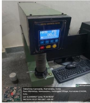
Figure 5: 5. Brinell hardness tester for testing of hardness of the composite
