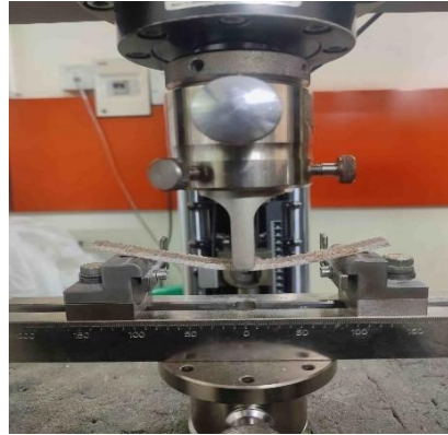
Figure 4: 4. Flexural test of bamboo-ramie hybrid composite
